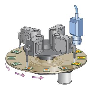
Rotary Indexers offer smooth motion, high load capacity and high speed. With their precision-grade, high-capacity cross-roller bearings, Rotary Indexers can handle loads up to 1,575 kilonewtons.
