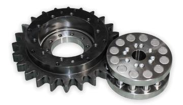
Nexen's Rotary Indexer System is based on the company's innovative Roller Pinion System (RPS) for linear motion. To create a Rotary Indexer, the linear rack becomes a circular Instead of moving a linear rack side to side, the pinion rotates the gear. The piniogeisr equipped with bearing-supported rollers that engage a unique tooth profile in the gear, providing smooth rolling friction instead of sliding friction.
