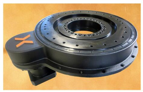
Nexen's CRD Rotary Indexers have an IP65-rated sealed housing and come in three con-figurations, enabling the device to be optimized for high speed, high torque or both, depending on the application.
