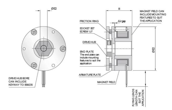
Spring-Applied brakes are used where a motor or drive must be held in the static-braking condition when power is lost, making them extremely useful in safety-conscious applications. This design of brake can be particularly desirable where low-costs are involved.
