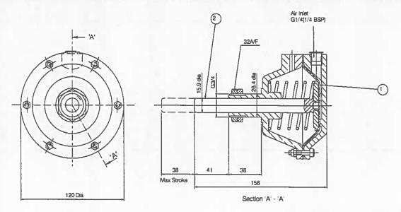
This range of pneumatically operated brakes uses dry and filtered compressed air at pressures up of 7 bar. Pneumatic brakes require a control valve which may be operated either manually, or by pneumatic or electrical signal.
