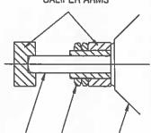
PUSHROD LOCKNUTS THRUSTER
