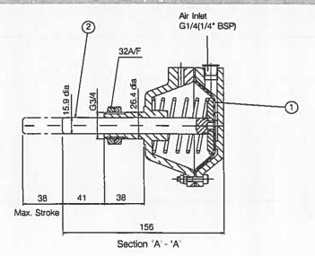
This range of pneumatically operated brakes uses dry and filtered compressed air at pressures up of 7 bar. Pneumatic brakes require a control valve which may be operated either manually, or by pneumatic or electrical signal.
