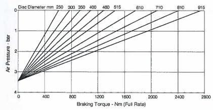
Weight (caliper and thruster) - 10.0kg (thruster only) - 3.5kg Total volume of air at full retraction is 0.95l
