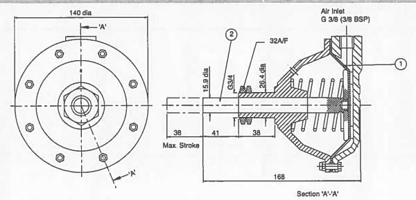
This range of pneumatically operated brakes uses dry and filtered compressed air at pressures up of 7 bar. Pneumatic brakes require a control valve which may be operated either manually, or by pneumatic or electrical signal.
