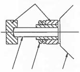
PUSHROD LOCKNUTS THRUSTER
